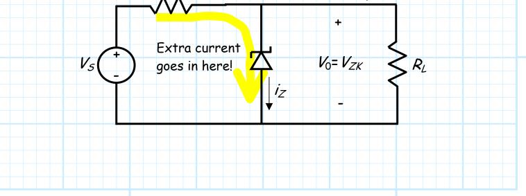
Similarly, if the load current  $i_L$  increases (i.e.,  $R_L$  decreases), then the Zener current  $i_Z$  will decrease by an equal amount. As a result, the current through shunt resistor R (and therefore the load voltage  $V_O$ ) will remain unchanged!
