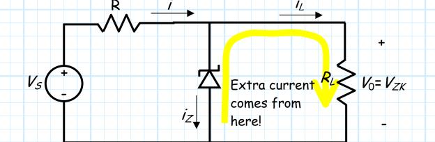
**Q**: You mean that  $V_O$  stays **perfectly constant**, regardless of source voltage  $V_S$  or load current  $i_L$ ??
